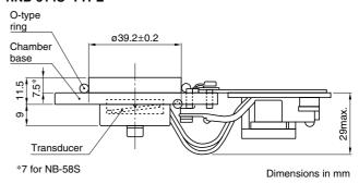
A 39.2mm diameter hole is formed in the bottom of the water chamber, which is connected using an O-type ring.
